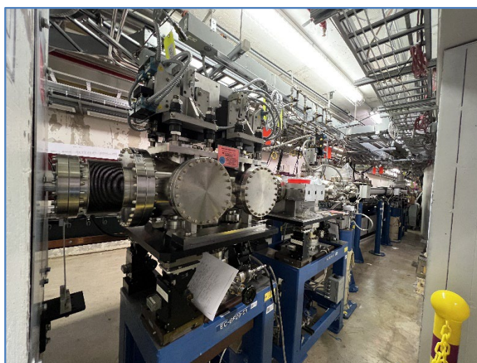
The APS storage ring tunnel at sector 23. Left: The APS storage ring and beamline front ends were removed by the end of June 2023. Right. The newly installed APS-U storage ring and sector 23 canted-undulator front end.
