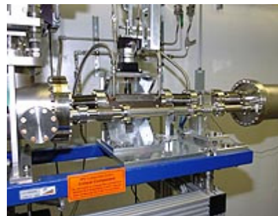
SPLIT BEAM – The two separate beamlines exit the cylinder at the right. They begin just hair widths apart and spread to two feet apart over the 60 meters they travel together. (Download hi-rez image .)
