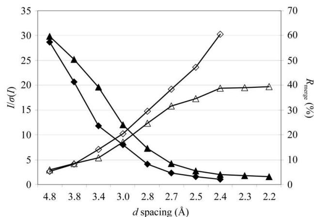
**Figure 3** Comparison of mini-beam and large-beam data from a needle-shaped crystal.  $I/\sigma(I)$  (solid symbols) and  $R_{\text{merge}}$  (open symbols) are plotted for data sets collected from a thioesterase crystal with the mini-beam (triangles; TENS) and with a large beam (diamonds; TENL). Owing to higher background and a poorer signal-to-noise ratio, the TENL data have a reduced effective diffraction limit and overall poorer statistics than the TENS mini-beam data.
